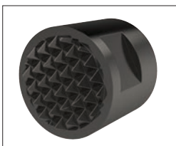
High Speed Tool Steel Manufactured from M-2 high speed tool steel, hardened to Rc 60/62 with black oxide finish. Mount via tapped hole, counter bored hole or a flat on the outside diameter for set screw mounting.
