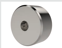
Stainless Steel Pad from 17-4 stainless steel, hardened to Rc 43/46. Mount via tapped or counter bored hole.
