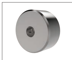
Hardened Steel Made from 8620 steel, carburized and hardened to Rc 58/60 1.2mm with black oxide finish. Mount via tapped or counter bored hole.
