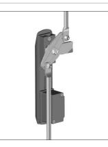
In conjunction with a standard cam latch, lock or swing handle, use a two point locking adapator A0243 and a latching rod set (A0303, A0321, A0325) to achieve two points of locking.
