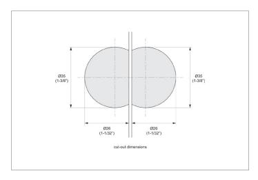
Max door thickness: 16-20mm. Overlay coverage: 14-16mm. Hinge alignment adjustable after installaton. Max. opening angle 90°.
