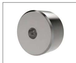
Hardened Steel Made from 8620 steel, carburized and hardened to Rc 58/60 1.2mm with black oxide finish. Mount via tapped or counter bored hole.
