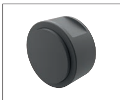
Carbide Tipped Constructed with high impact carbide pad brazed to a heat treated alloy steel body. Mount via tapped hole or a flat on the outside diameter for set screw mounting.
