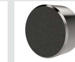
Abrasive Diamond Surface Abrasive surface permanently fused to a 17-4 stainless steel pad, hardened to Rc 43/46. The surface texture is comparable to a 100 grit abrasive. Mount via tapped or counter bored hole.
