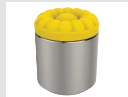
Soft Urethane Surface Urethane surface is permanently bonded to a 300 series stainless steel pad. The urethane provides excellent protection against damage on delicate work surfaces. Tapped hole mounting.
