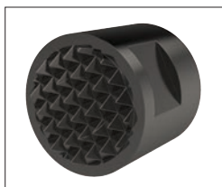
High Speed Tool Steel Manufactured from M-2 high speed tool steel, hardened to Rc 60/62 with black oxide finish. Mount via tapped hole, counter bored hole or a flat on the outside diameter for set screw mounting.
