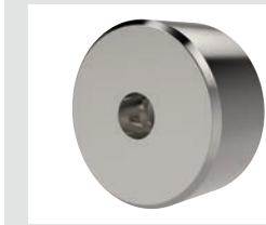
Stainless Steel Pad from 17-4 stainless steel, hardened to Rc 43/46. Mount via tapped or counter bored hole.
